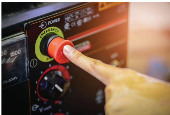
Figure 13 - Machine with Emergency Stop Switch.
