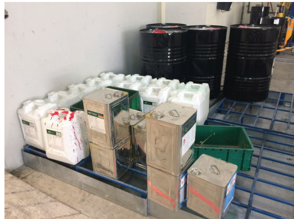
Figure 19 - Chemical Storage Room with Secondary containment device.
