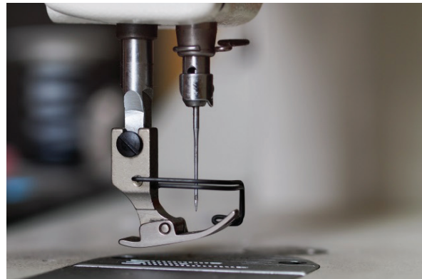
Figure 11 - Proper Needle Guarding on a Sewing Machine
